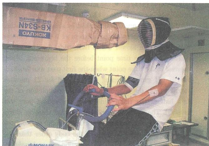
**Fig.1:** The situation of an experiment. All the subjects measured with the bicycle ergometer, after putting a kendo *men* in the climatic chamber.
