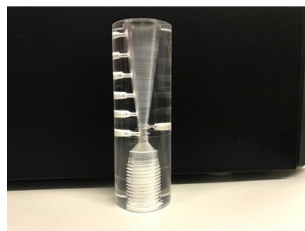
Fig.2 Nozzle photograph used in experiment ( \theta=11 [°])
