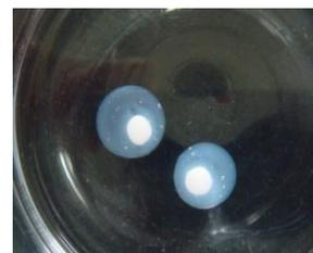
Fig. 6 Photograph of alginate shell formed around the chitosan core.
