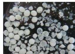
Fig. 5 The chitosan core after crosslinking by glutaraldehyde for over 10 min..
