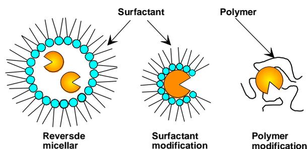
Fig.1 Schematic diagram of modifying methods of enzyme.
