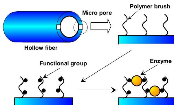
Fig.2 Schematic diagram of lipase immobilized onto the pores of hollow fiber.
